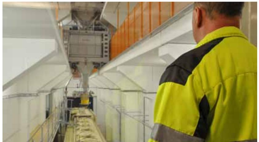
The end product goes to one of the 96 finished product silos. There are three loading lanes for bulk trucks. Each loading station is equipped with a double robot weigher for maximum speed and flexibility.
